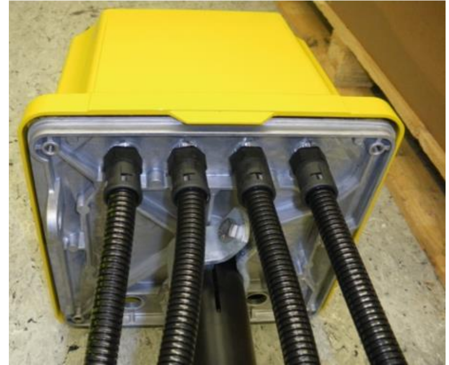
Signal junction box
