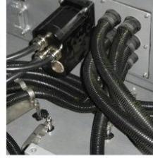
As a result, tough PH410EX conduits with PH400 polyamide sleeves are used on the roof and underframe applications. The PH400 sleeves are designed to withstand temperatures that run through couplings to the bridge.
